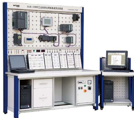
DLGK-SIMND 工業自動化網路集成實訓系統 Industrial Automation Network Integration Training System
